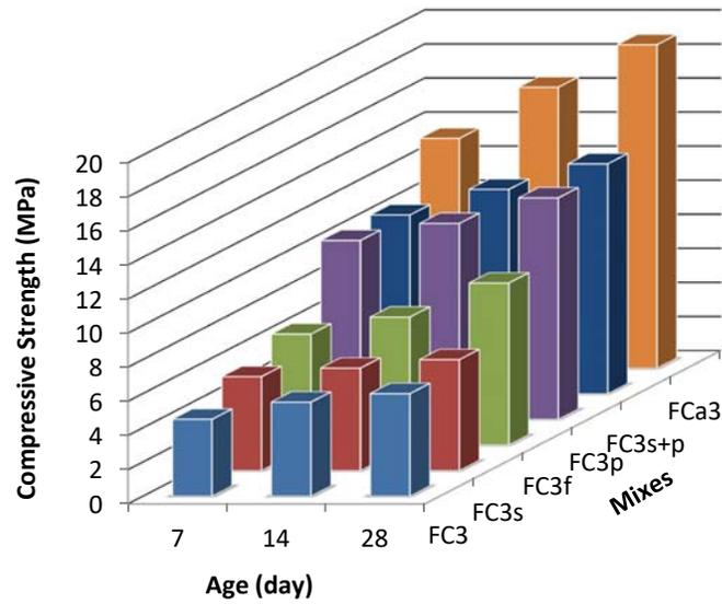
546 **Fig. 1.** Effect of used additives on the compressive strength of 1300 kg/m<sup>3</sup> mix.
