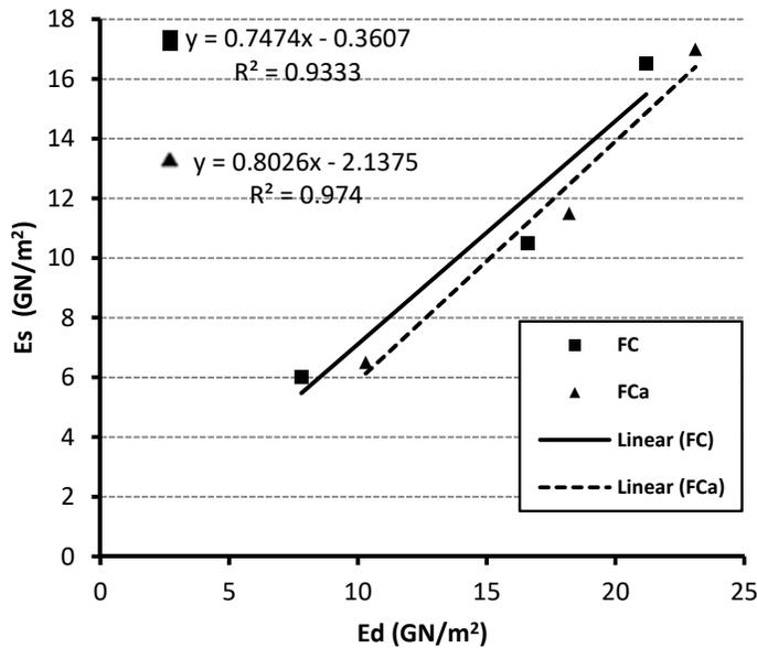
**Fig. 13.** Relationship between static and dynamic modulus of elasticity at 28 day of foamed concrete mixes.
