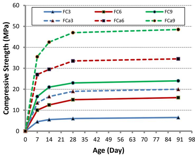
589 **Fig. 6.** Development of 100mm cube sealed-cured compressive strength.
