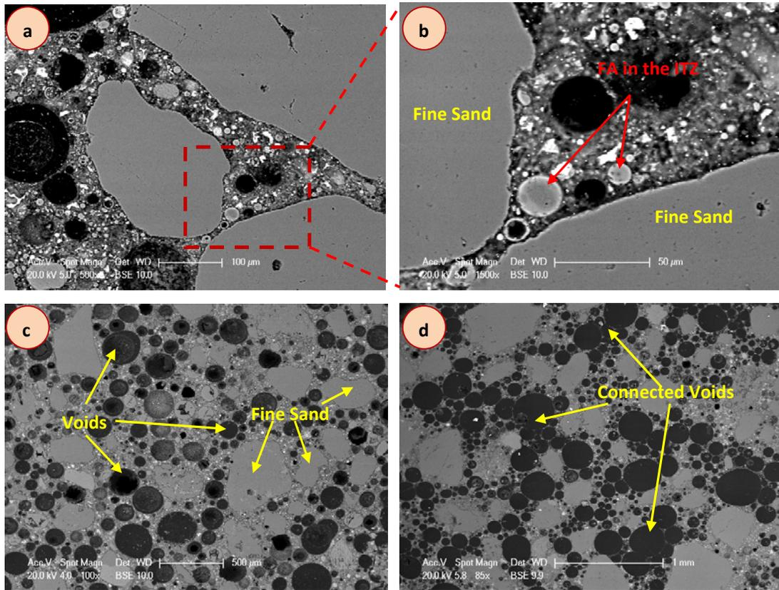
**Fig. 7.** Scanning Electron Microscopy images of 1300 kg/m<sup>3</sup> foamed concrete (a, b and c) with additives (FCa3), (d) conventional.
