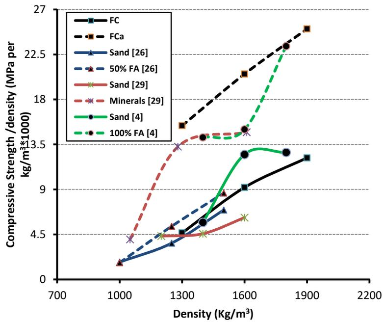
**Fig. 8.** Strength to density ratios for different foamed concrete mixes.
