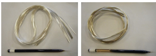
Figure 2: Fibre production from extruded core/clad preforms. Fibres were drawn with diameters ranging from 30–50 \mu\text{m} .
