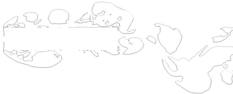
Figure 12. Contour of Q = 0.1\text{ms}^{-1} along the mid-span plane at U_r = 2.83 .
