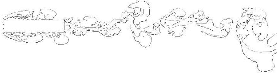
Figure 19. Contour of Q = 0.1 \text{ ms}^{-1} along the plane at y/D = 0 (the static end).
