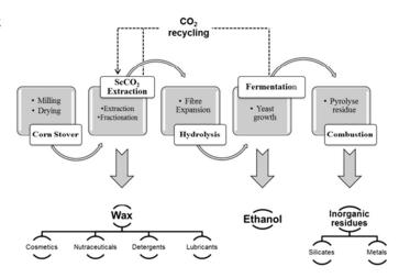
Figure 10 Concept of holistic maize stover biorefinery with scCO<sub>2</sub> as a pre-treatment step.
