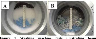
Figure 5 Washing machine tests illustrating foam generation A) Control Run B) Run with Wax.
