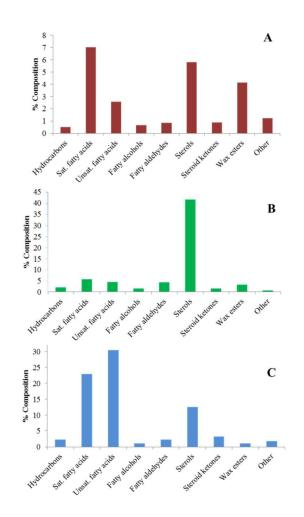
Figure 3 Composition of groups of compounds for each wax fraction A (400-150 bar/50 °C) B (150-80 bar/35 °C) C (80-ATM/ 50°C)
