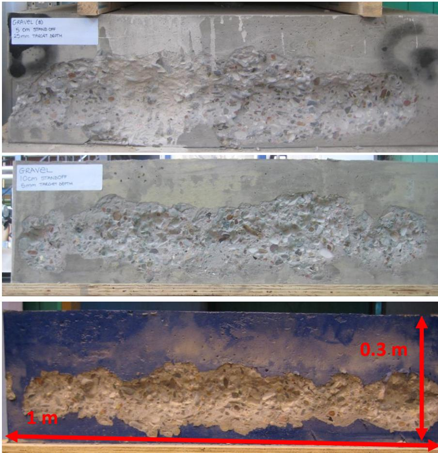
Figure 15: Effect of stand-off distance and painting the gravel-based concrete surface post treatment at 15kW (50mm stand-off – top, 100mm standoff – middle, painted surface 50 mm stand off – bottom)
