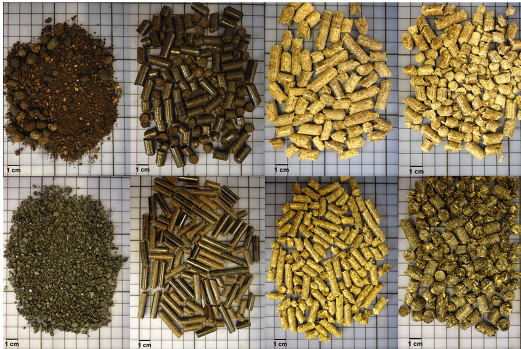
Fig. 1. (top left to right) Spanish olive cake, torrefied pellets, wood pellets, South African eucalyptus pellets, (bottom left to right) Colombian La Loma coal, steam exploded pellets, miscanthus pellets, sunflower husk pellets.
