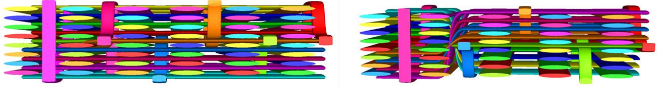
Figure 7. As-woven textile models. Left, Variation I; Right, Variation II
