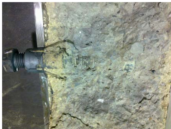
Fig. 9. Specimen after fire exposure.
