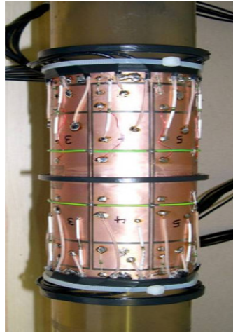
Figure 2: Photo of the Electrical Capacitance Tomography (ECT)
