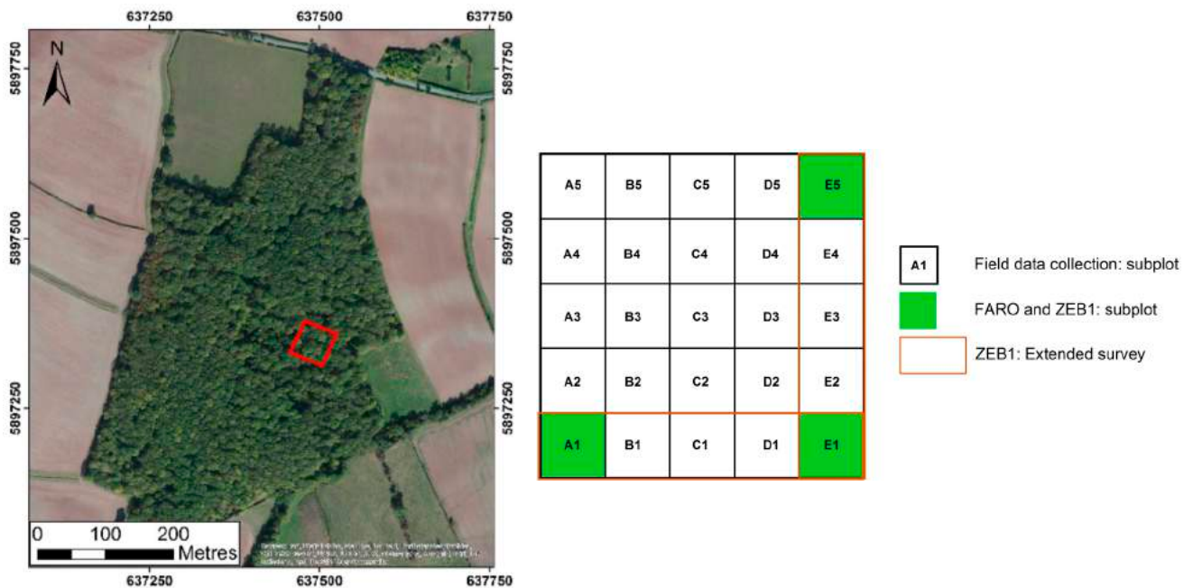
Figure 2. Kirton Wood survey plan showing location of test site within woodland and subplot position (image source: Esri, DigitalGlobe, GeoEye, i-cubed, Earthstar Geographics, CNES/Airbus DS, USDA, USGS, AEX, Getmapping, Aerogird, IGN, IGP, swisstopo, and the GIS User Community).
