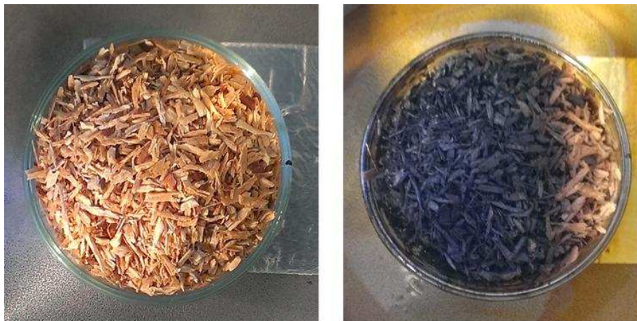
Figure 8 – Images of 20g untreated sample (left) and sample treated at 1kW and 500 kWh/t (right)
