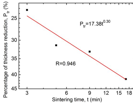
Fig. 6 Plot of percentage of thickness reduction versus sintering time on log-log coordinates.
