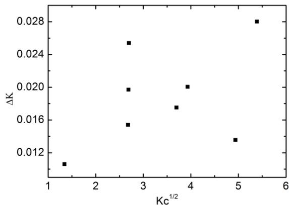
Fig. 11 Willimson-Hall plot obtained from the XRD spectrum of the sample sintered for 5 minutes.
