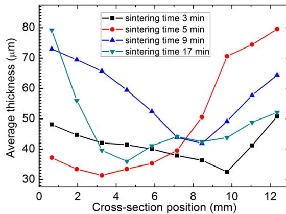
Fig. 4 Plots of thickness versus cross-sectional position for the four samples of attaching Si IGBTs on Si<sub>3</sub>N<sub>4</sub>-based substrates.
