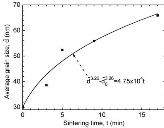
Fig. 14 Plot of average grain size versus sintering time on linear coordinates.
