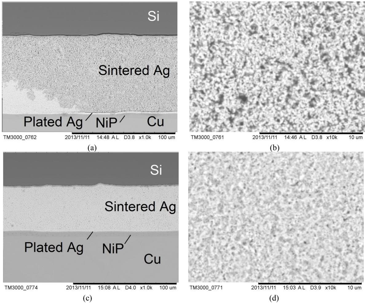
Fig. 3 SEM images taken from the polished and plasma-etched cross section of the sample of attaching one Si IGBT on the Si<sub>3</sub>N<sub>4</sub>-based substrate at 240°C and 5 MPa for 9 minutes: (a) overview at edge area; (b) enlarged view at edged area; (c) overview in the central area; and (d) enlarged view in the central area.
