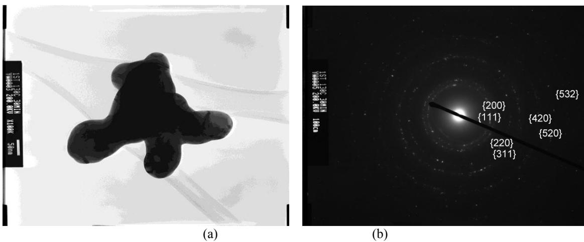
Fig. 12 TEM results of the as-dried paste of Ag nanoparticles: (a) one TEM image and (b) the corresponding electronic diffraction rings for multiple Ag grains.
