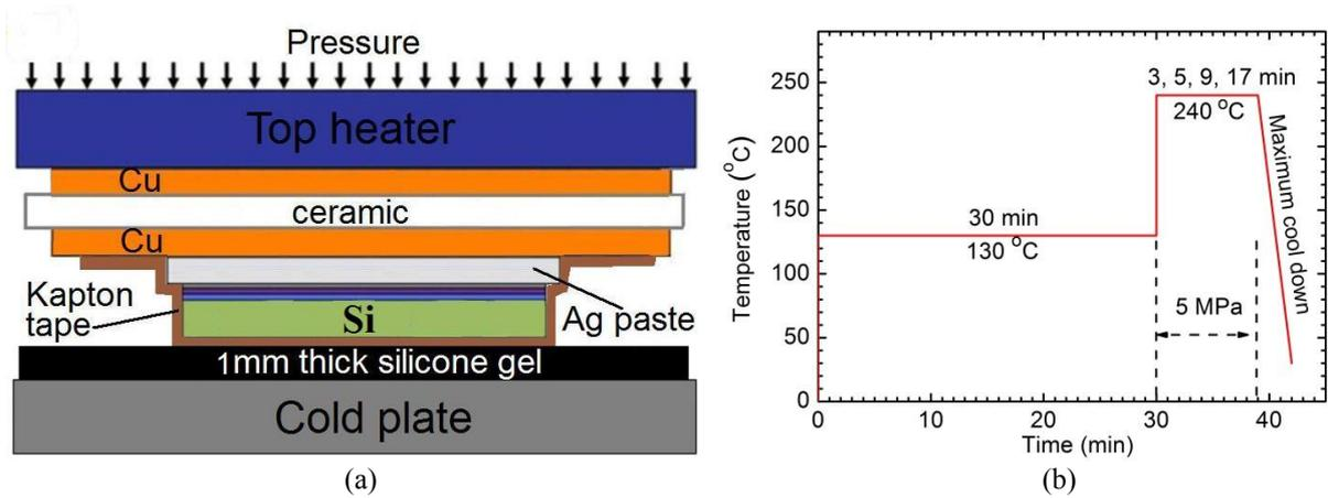
Fig. 1 Schematic diagrams of (a) sample geometry and (b) temperature and pressure profile used during the sintering process. Note that the dimensions of sample geometry are not to scale.
