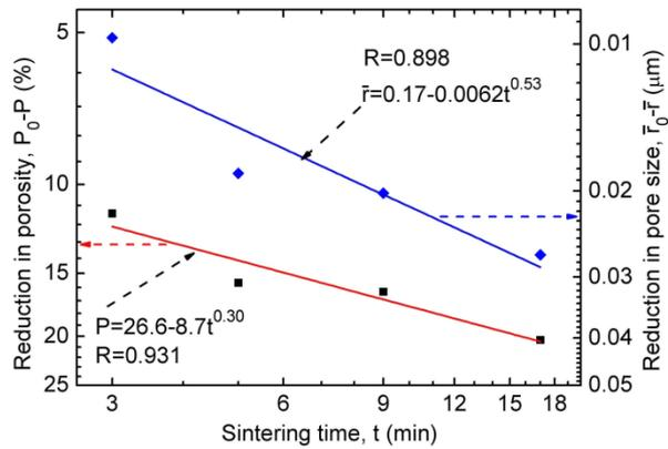
Fig. 9 Plots of reductions in pore size and porosity versus sintering time on log-log coordinates.
