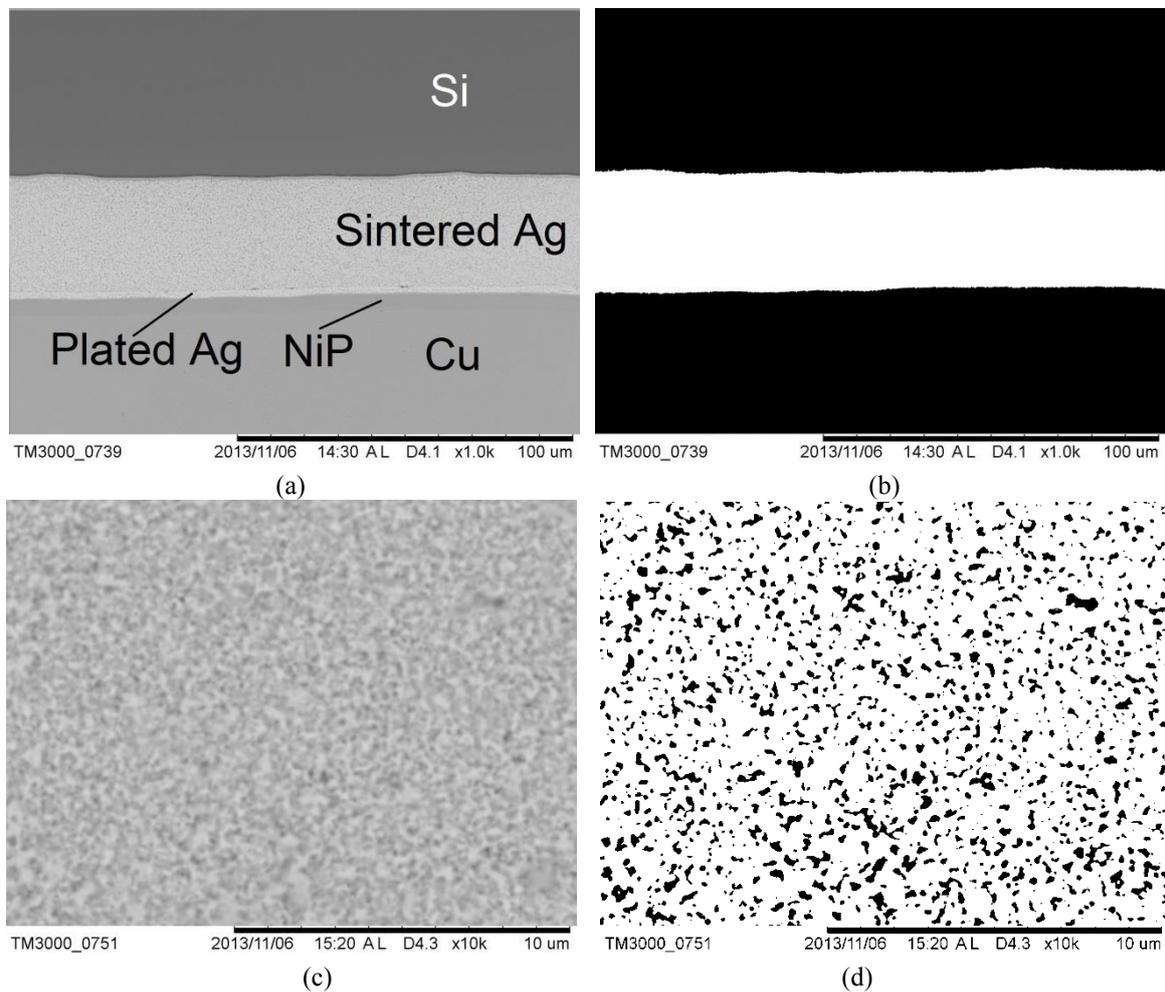
Fig. 2 (a) One representative SEM image and (b) the corresponding black and white binary used to measure the thickness values; (c) one representative SEM images and (d) the corresponding black and white binary used to measure the pore size and porosity values for the sample of attaching one Si IGBT on the  $\text{Si}_3\text{N}_4$ -based substrate at 240°C and 5 MPa for 5 minutes.
