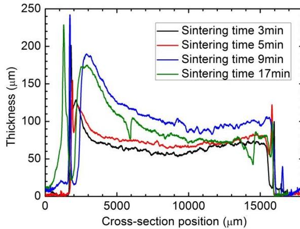
Fig. 5 Plots of thickness versus central cross-sectional position measured with a surface profiler for the four pads of paste of Ag nanoparticles printed on the  $\text{Si}_3\text{N}_4$ -based substrates which were dried at  $130^\circ\text{C}$  for 30 min prior to attaching the Si IGBTs on them at  $240^\circ\text{C}$  and 5 MPa for 3 to 17 minutes.
