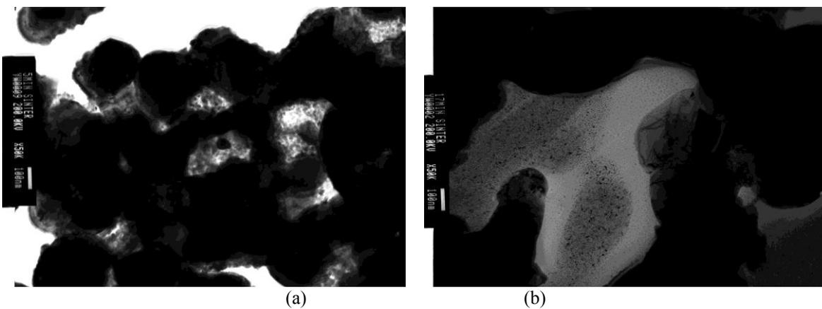
Fig. 13 TEM images taken from the samples sintered for: (a) 5 min and (b) 17 min.
