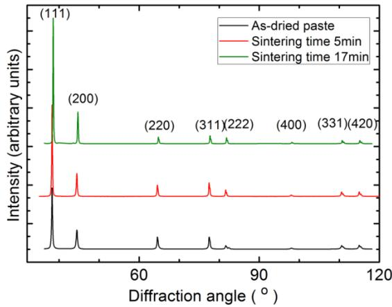
Fig. 10 XRD spectra of the as-dried paste of Ag nanoparticles and the samples sintered for 5 and 17 minutes.
