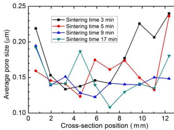
Fig. 7 Plots of average pore size versus cross-section position for the four samples of attaching Si IGBTs on  $\text{Si}_3\text{N}_4$ -based substrates.
