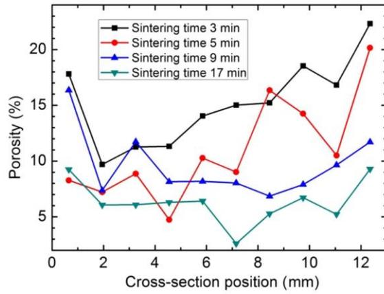
Fig. 8 Plots of porosity versus cross-section position for the four samples of attaching Si IGBTs on Si<sub>3</sub>N<sub>4</sub>-based substrates.
