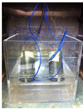
Figure 5 Photographs and schematic diagram for the rapid chloride migration test
