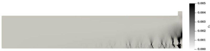
288 Figure 6 Crack pattern of beam at 100% peak load in terms of maximum principal strain.
