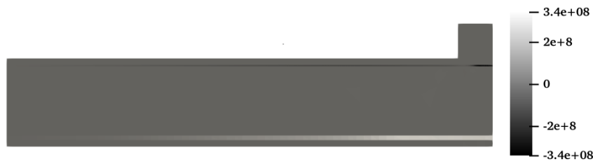
295 Figure 7 Axial stresses ( \text{N/m}^2 ) in longitudinal bars at peak force.
