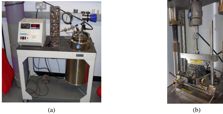
Fig. 1. (a) Saturation Ageing Tensile Stiffness (SATS) conditioning equipment [12]. (b) Indirect Tensile Stiffness Modulus (ITSM) setup in Nottingham Asphalt Tester (NAT) machine.
