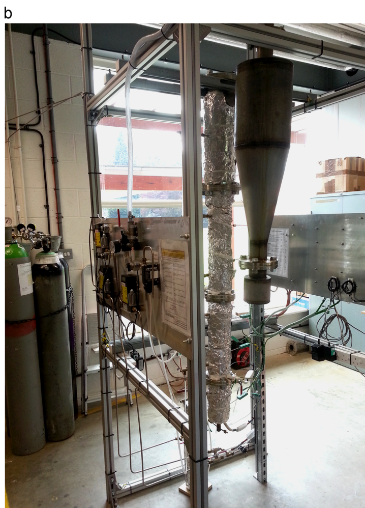
Fig. 1. Schematic and photograph of the bubbling fluidized bed reactor.
