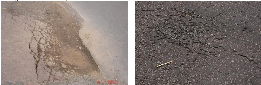
Fig. 2. Different Examples of Road Distress Types: (a) Pothole Distress; (b) Cracking Distress
