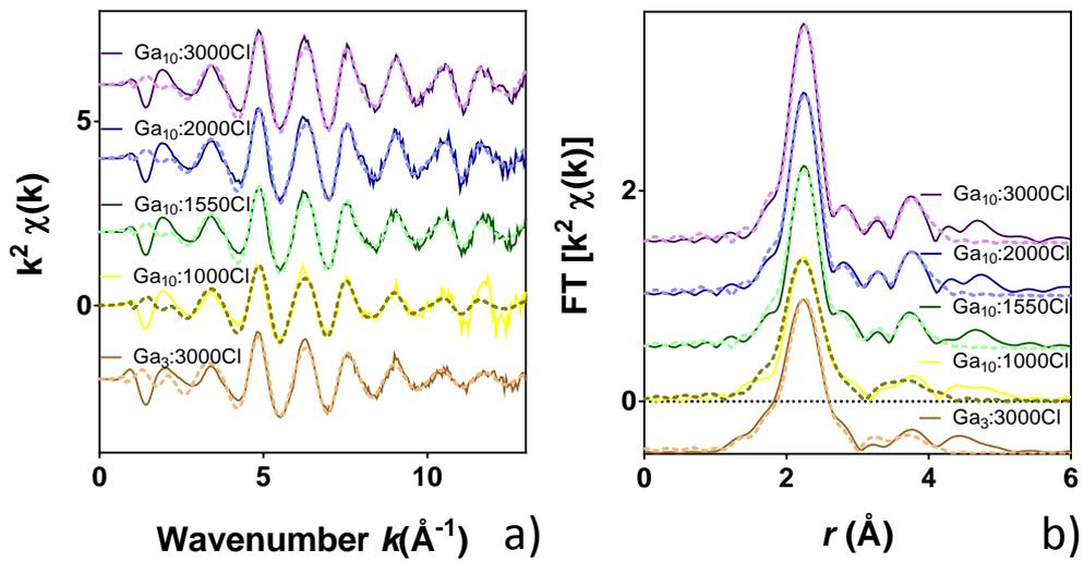
Figure 6: EXAFS fits in: a)  $k^2$  and b) real space, for the  $\text{Ga}_{10}:1000\text{Cl}$ ,  $\text{Ga}_{10}:1550\text{Cl}$ ,  $\text{Ga}_{10}:2000\text{Cl}$ ,  $\text{Ga}_{10}:3000\text{Cl}$ , and  $\text{Ga}_3:3000\text{Cl}$  glasses. Experimental data are shown with a solid line and dashed lines show the fit.
