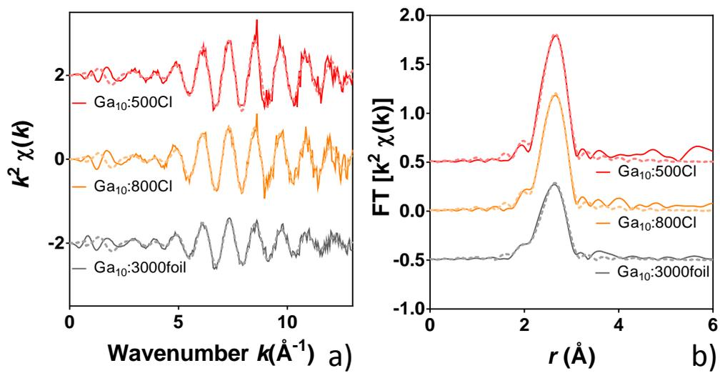
Figure 5: EXAFS fits in: a)  $k^2$  and b) real space, for the Ga<sub>10</sub>:3000foil, Ga<sub>10</sub>:500Cl and Ga<sub>10</sub>:800Cl glasses. Experimental data are shown with a solid line and dashed lines show the fit.
