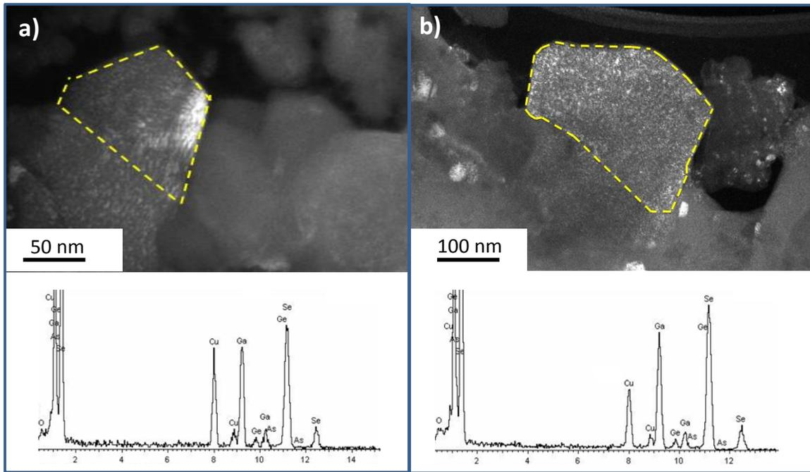
Figure 2: HRTEM images for: a) Ga<sub>3</sub>:3000Cl [11] and b) Ga<sub>10</sub>:2000Cl [12], with an  $\alpha$ -Ga<sub>2</sub>Se<sub>3</sub> crystal highlighted (yellow dashed line). The elemental analysis of the crystal phase is also shown [11].
