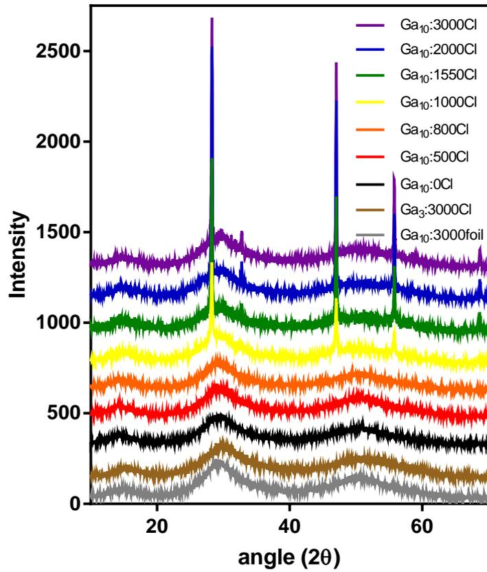
Figure 1: X-ray diffraction patterns measured for nine glasses of composition  $\text{Ge}_{16.5}\text{As}_9\text{Ga}_{10}\text{Se}_{64.5}$ (at%) doped with 0 to 3000 ppmw  $\text{Dy}^{3+}$  [7,11,12,19,20]. The X-ray patterns are offset on the y-axis for clarity.
