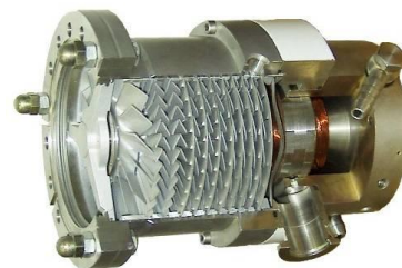
Fig. 6. Cross-section of turbomolecular pump driven by high speed motor [76]
