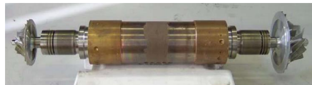
Fig. 16. 300kW 60,000 rpm copper coated solid rotor IM, Sundyne Corp. [30]
