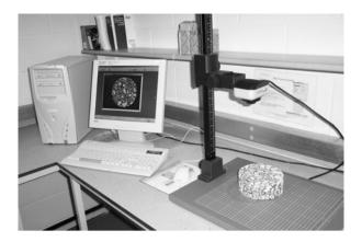
Figure 1. 2D image analysis equipment.
