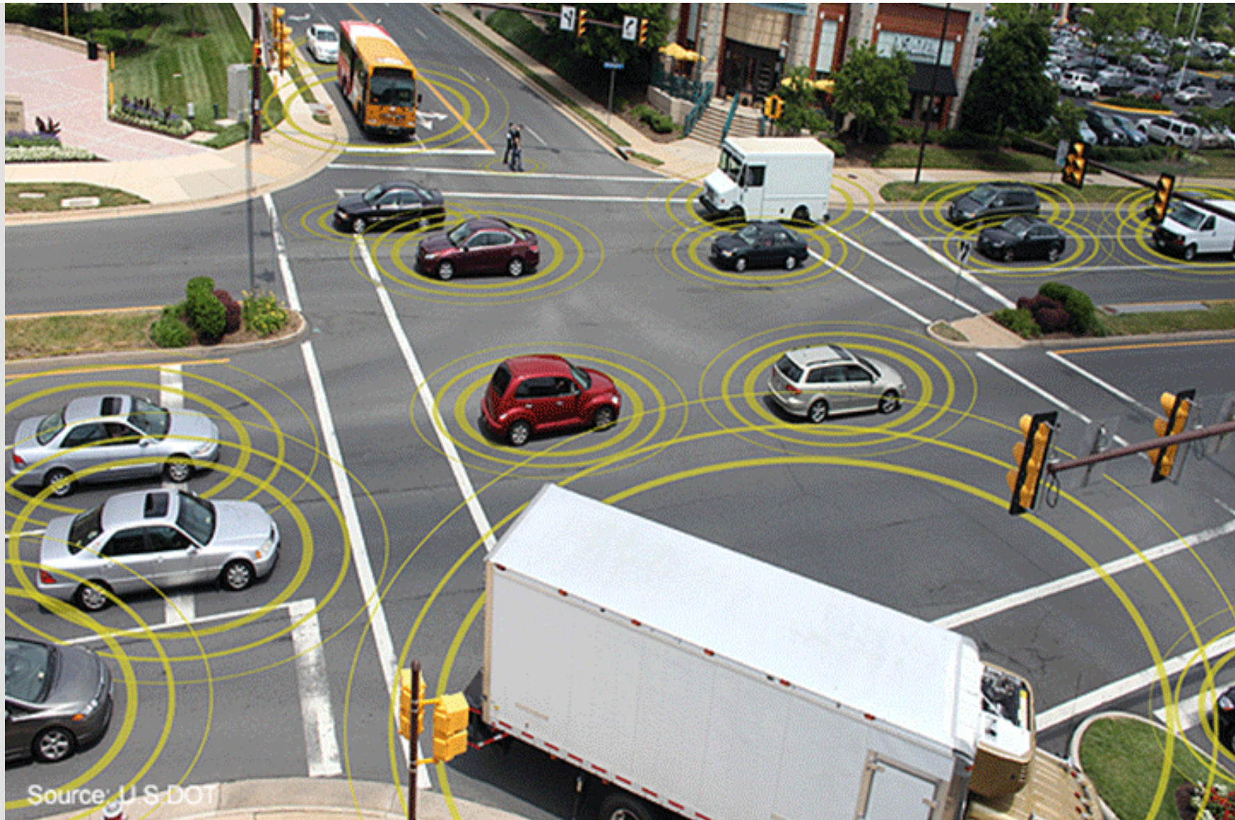
□ Figure 1. Vehicle-to-vehicle communications as envisioned by the United States Department of Transportation.
