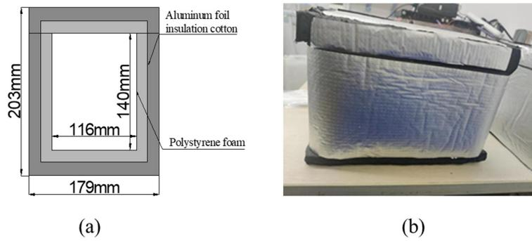
Fig. 10. (a) The cross section of box, (b) Photograph of the insulated box.
