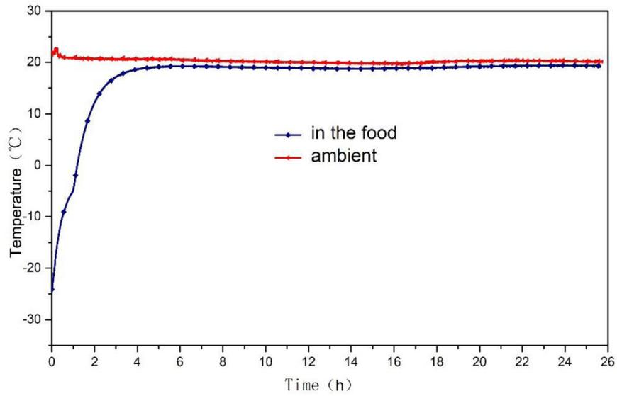
Fig. 11. Temperature varied with time for insulated box without PCM.
