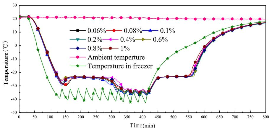
Fig. 8. Temperature variation of SPW gel added with different ratios of TiO<sub>2</sub> during solidification process and melting process.
