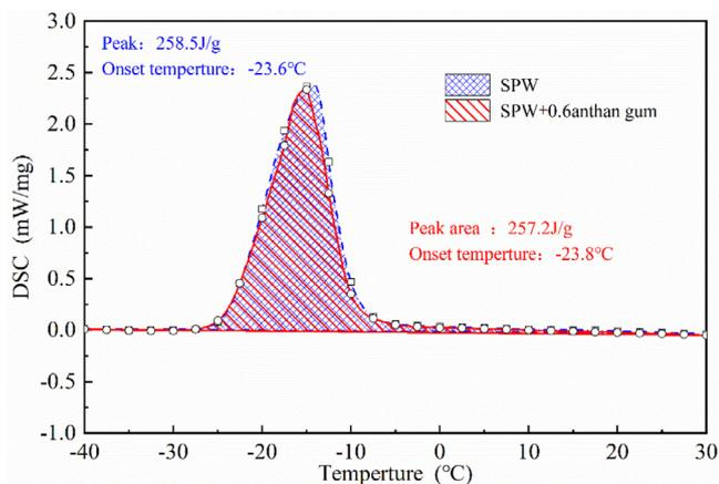
Fig. 7. Comparison of DSC tests for SPW fluid and SPW gel.
