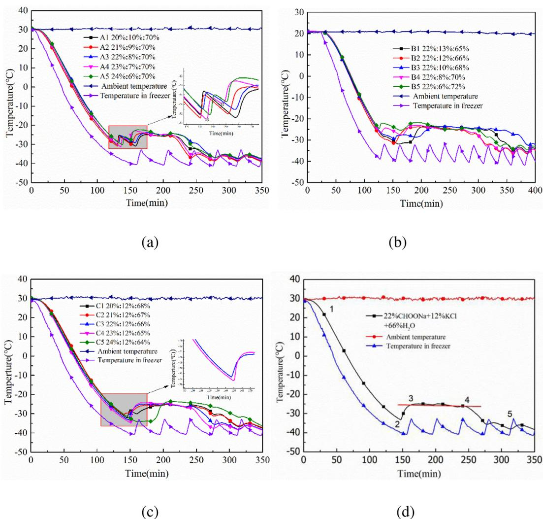
Fig. 2. The cooling curves of different proportions SPWs of (a) group A in Table 2, (b) group B in Table 3, (c) group C in Table 4, (d) C3 sample (22%:12%:66%).
