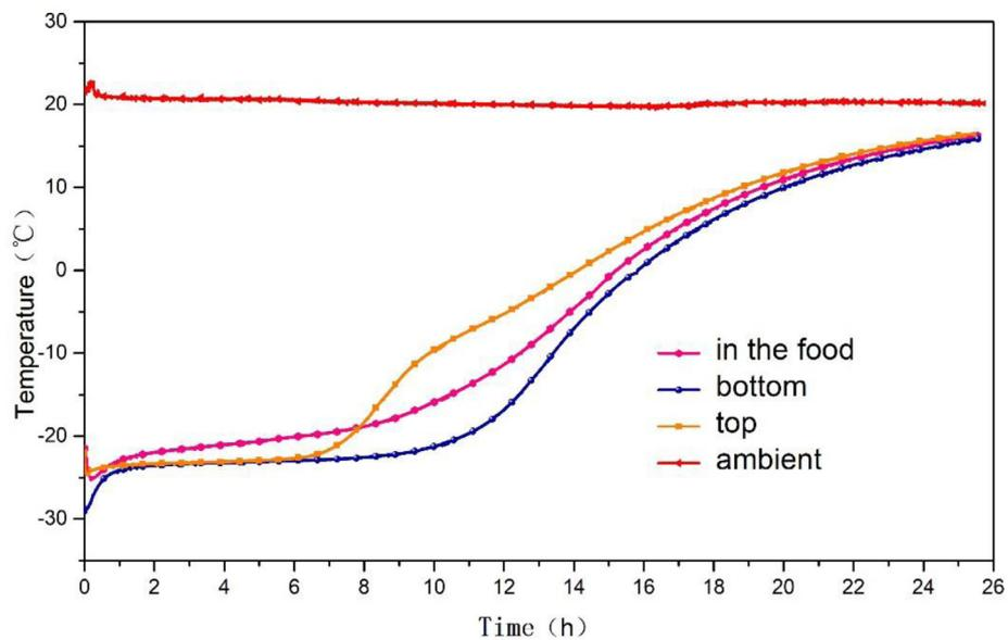
Fig. 12. Temperature varied with time for insulated box with PCM.
