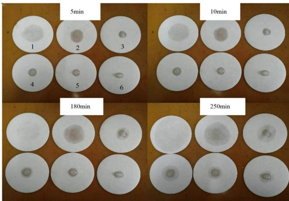
Fig. 6. Flow performance of SPW added with different mass fractions of xanthan gum.
