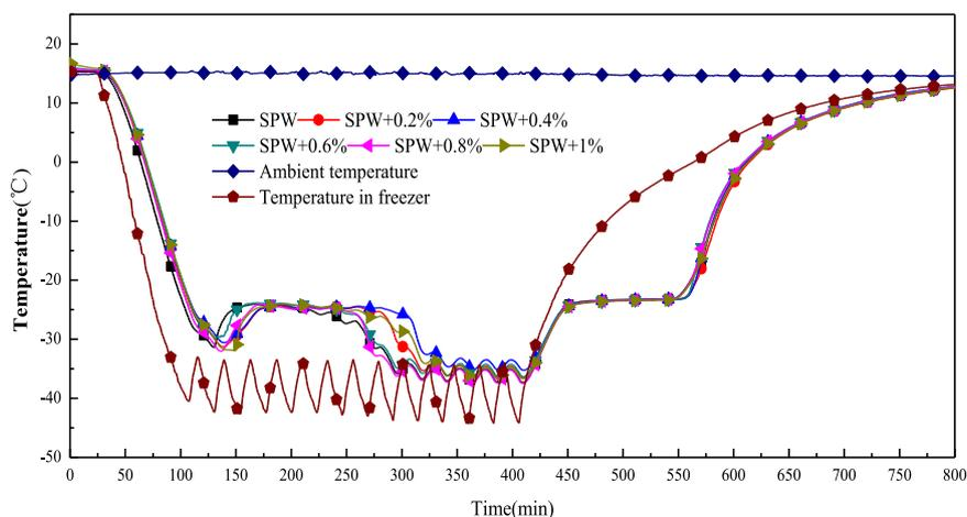
Fig. 4. Temperature variation of SPW composites with different ratios of xanthan gum during solidification process and melting process.
