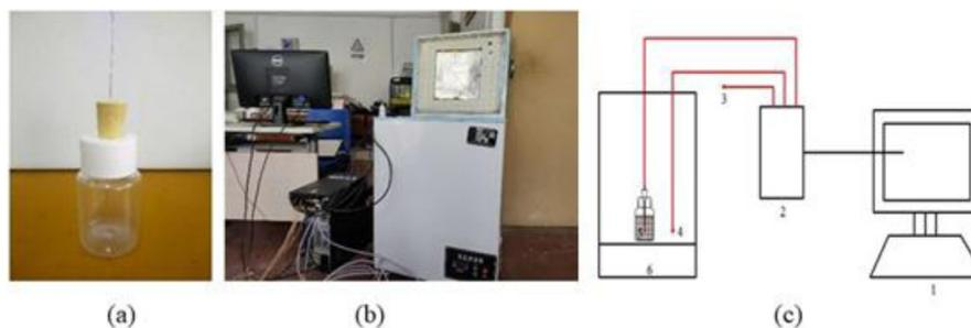
**Fig. 1.** (a) Photo of the plastic sample vial, (b) Photo of experimental equipment, (c) Schematic diagram of experimental system (1. Computer, 2. Data acquisition board, 3. Ambient temperature, 4. Temperature in freezer, 5. Sample temperature, 6. Freezer).
