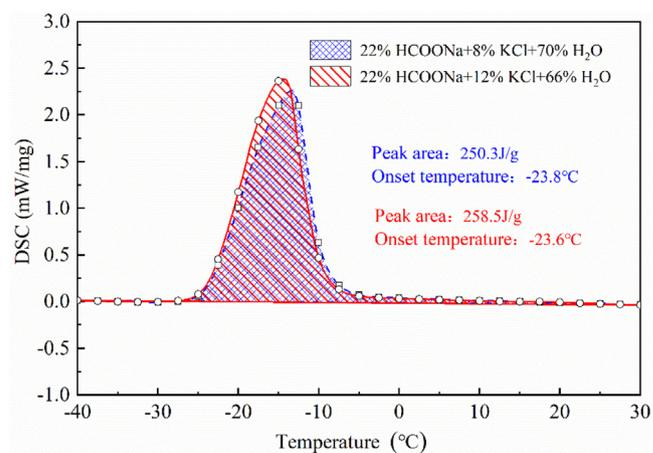
Fig. 3. DSC results of cooling test-selected SPW and DSC-selected SPW (Lu et al., 2019).
