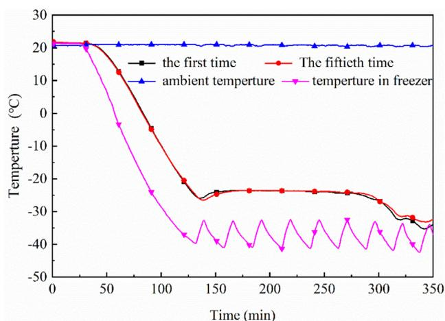
Fig. 9. Cooling curves of SPW composite before and after life cycles.
