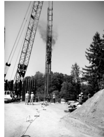
Figure 12 – Ground surface geophones on line with pile being driven
