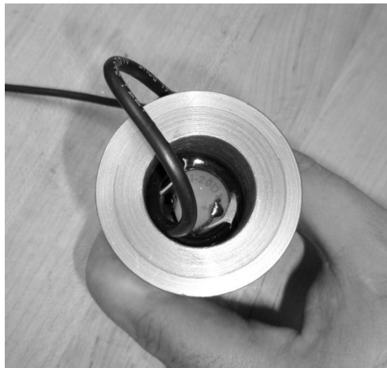
Figure 6 – Geophone potted in push cone cavity
