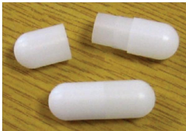
**Figure 2** Magnetic resonance imaging (MRI) marker capsule. Example of a capsule which consists of two polyoxymethylene half shells glued together, and hand filled with 0.4 mL 15 μM Gadoteric acid (Gd-DOTA). Leakage tests performed on 20% of each batch using a spectrophotometer. Capsules have the dimensions of 20 × 7 mm.
