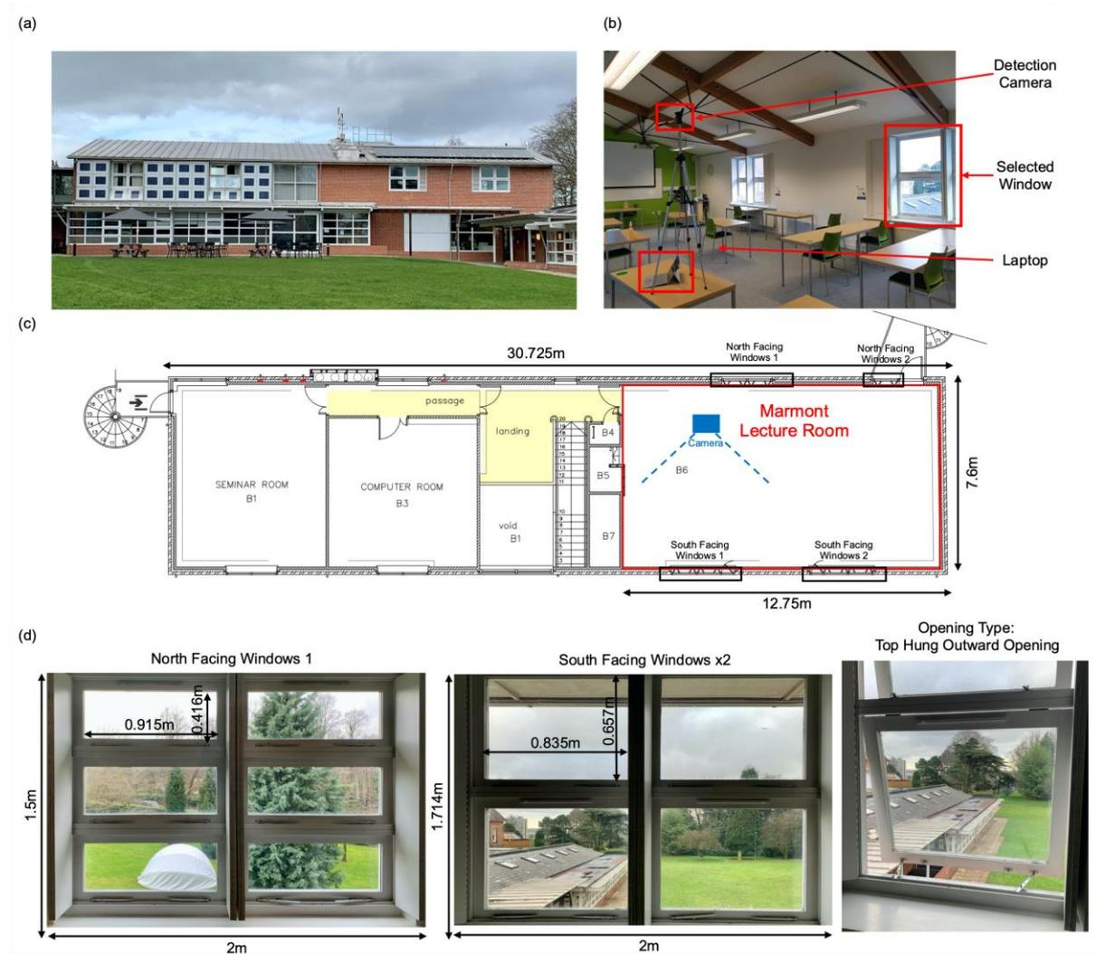
Figure 2. (a) Marmont Centre at the University of Nottingham, UK. (b). Set up for the experimental test. (c). 1<sup>st</sup> Floor plan. (d) Design and configuration of windows within the Marmont lecture room.
