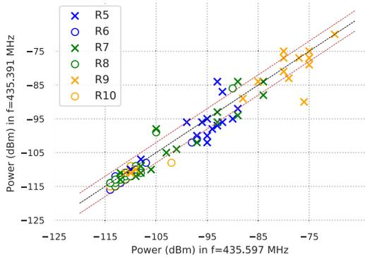
(c) Distribution of power over close carriers. The black dashed line showed the tendency if the power in one carrier was completely dependent on the other and the red dashed lines, a difference of  $\pm 3$  dB.
