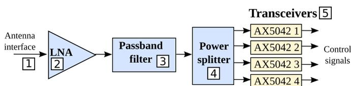
(a) RF payload architecture based on the diagram from (Muñio & Agelet, 2014).
