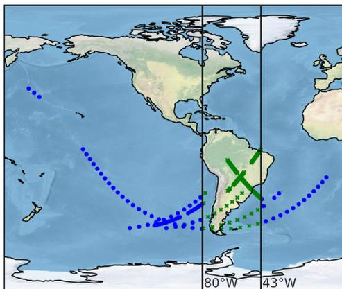
(a) Sub-satellite points for measurements over several orbits over the ocean (blue circles) and South America (green crosses). For each point there were four power values, one per frequency.
