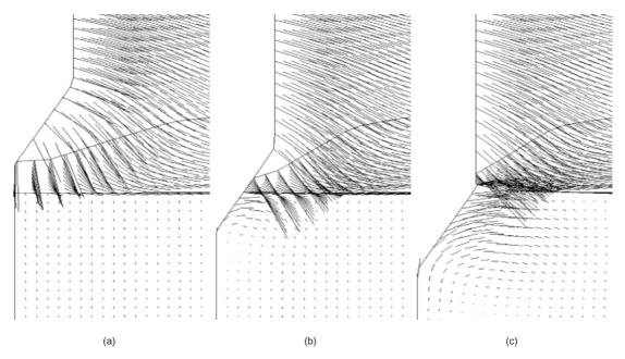
Fig. 17. The displacement field around the cone
