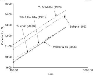
Fig. 1. Comparison of cone factors from various analyses
