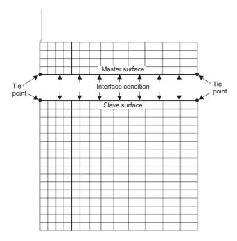
Fig. 3. Boundary constraints and interface conditions
