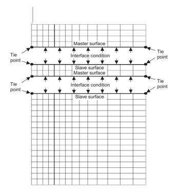
Fig. 11. Boundary constraints and interface conditions
