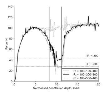
Fig. 13. Penetration resistance in a multi-layered soil
