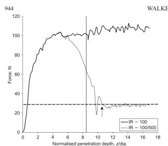
Fig. 9. Penetration resistance in a dual-layered soil
