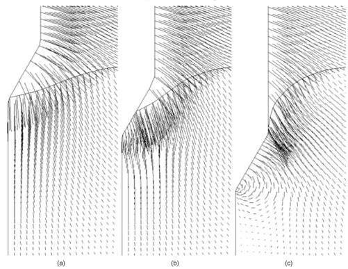
Fig. 5. The displacement field around the cone
