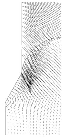
Fig. 8. The displacement field around the cone
