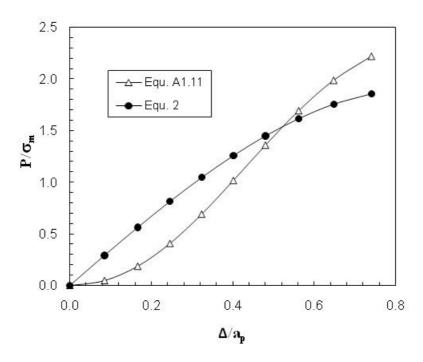
Fig. 12(b) Variations of P/ $\sigma_m$  with  $\Delta/a_p$ , for  $a_p$  = 2mm,  $R_s$  = 1.25mm and  $t_o$  = 0.5mm.
