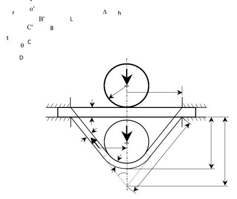
Fig. 4 Initial and deformed (assumed constant thickness) shape of the SPT specimen.
