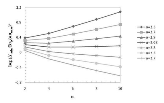
Fig. 36 Variations of log[ $(\dot{\Delta}_{min})$ / Ba $_p(\alpha\sigma_{nom})^n$ ] with n for various  $\alpha$ -values.
