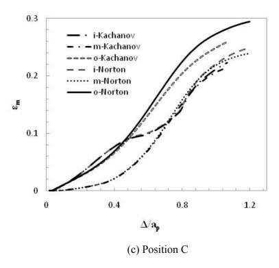
Fig. 31  $\epsilon_m$  versus  $\Delta$  at inside, i, middle, m, and outside, o, for both Kachanov damage model and Norton's law.
