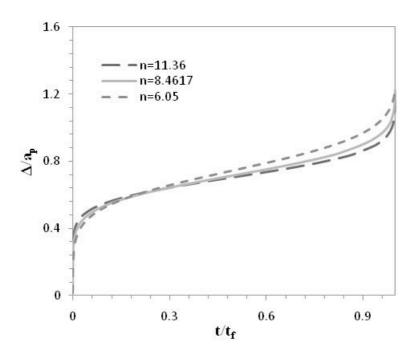
Fig. 21  $\Delta$  versus  $t_{\rm f}$  for Norton law creep behaviour with n=6.05, 8.4617, 11.36.
