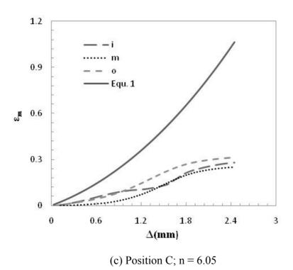
Fig. 22  $\epsilon_m$  versus  $\Delta$  at inside, i, middle, m, and outside, o.
