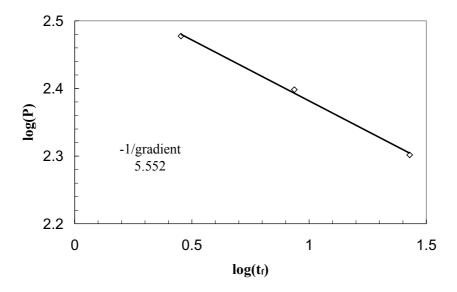
Fig. 33 FE predictions of log (P) versus log ( $t_{\rm f}$ ) based on Kachanov damage model.
