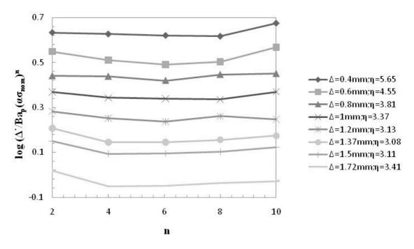
Fig. 37 Variations of log  $(\dot{\Delta}\dot{\Delta}/Ba_p(\eta\sigma_{nom})^n)$  with n for various of  $\Delta$ -values for the  $\alpha$ -values which produce approximately horizontal lines (N.B. for this condition  $\alpha = \eta$ ).
