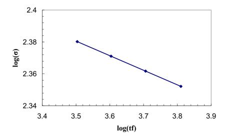
Fig 16 Creep rupture data for a brittle (Kachanov damage) failure model using constants for 316 stainless steel at  $600^{\circ}$ C (gradient =  $-1/\chi$ )
