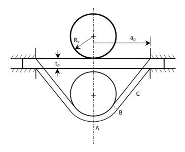
Fig. 3(a) Schematic diagram of typical SPT setup.
