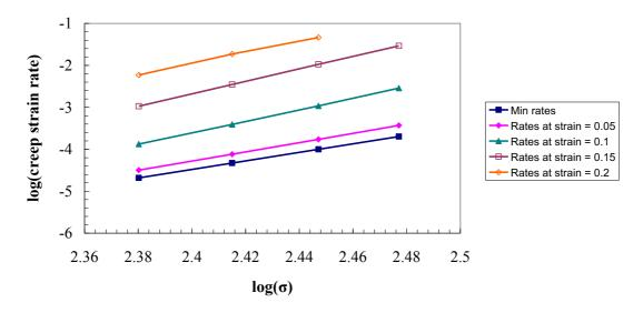
Fig 18(a) Creep strain rate vs.  $\sigma$  on a log-log scale using the Liu and Murakami damage model (for 316 stainless steel at 600°C)
