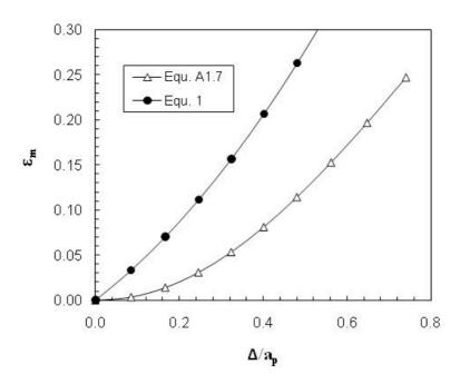
Fig. 12(a) Variations of  $\epsilon_m$  with  $\Delta/a_p$  for  $a_p$  = 2mm and  $R_s$  = 1.25mm.
