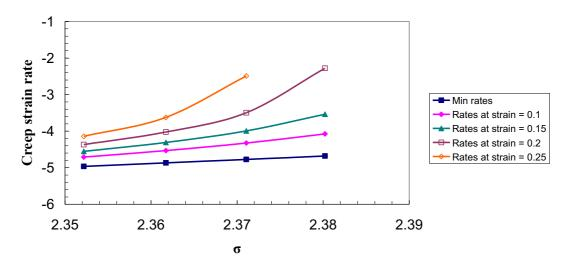
Fig 19(a) Creep strain rate vs.  $\sigma$  on a log-log scale using the Kachanov damage model (for 316 stainless steel at 600°C)
