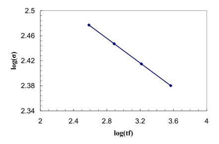
Fig 14 Creep rupture data for a ductile (Norton creep law) failure model, based on constants for 316 stainless steel at  $600^{\circ}$ C (gradient = -1/n)
