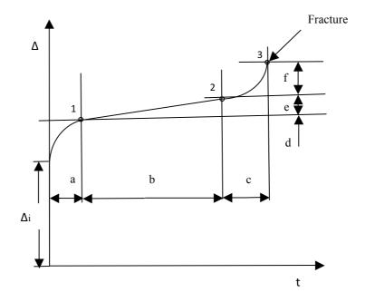
Fig. 3(b) Schematic representation of displacement versus time curve from SPT showing different deformation regions(where Δ<sub>i</sub> is the instantaneous elastic and plastic deformation):
