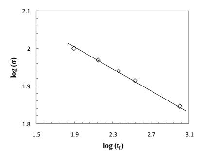
Fig. 1 (a) Typical conventional creep test specimen (GL  $\approx$  50mm, $d_{GL}$   $d_{GL}$   $\approx$  10mm); (b) Uniaxial creep strain curves for a P91 steel at 650° C; (c) Creep rupture data for a P91 steel at 650° C.
