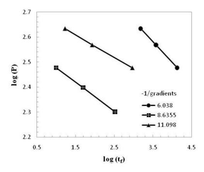
Fig. 27 FE predictions of log (P) versus log ( $t_f$ ) based on Norton's law (n = 6.05; n = 8.4617; n = 11.36).
