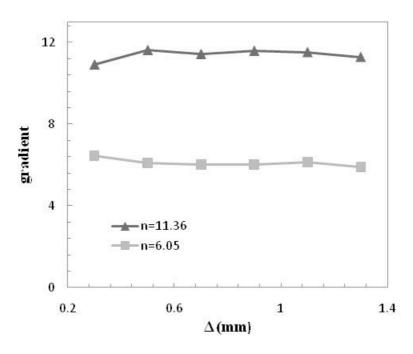
Fig. 29 Variation of gradient (of log  $(\dot{\Delta})$  versus log (P)) with  $\Delta$ .
