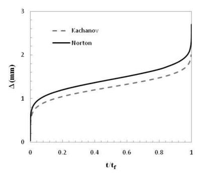
Fig. 30 Comparison of  $\Delta$  versus  $t/t_f$  for both Kachanov damage model and Norton's law.
