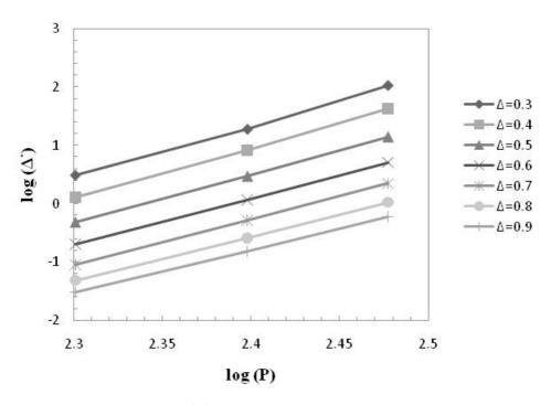
Fig. 34 FE predictions of  $log(\dot{\Delta})$  versus log(P) based on Kachanov damage model for different  $\Delta$  values.
