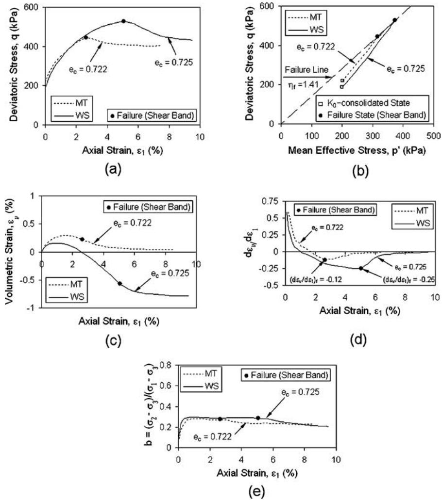
FIG. 6—Comparison of drained tests conducted on WS and MT specimens.
