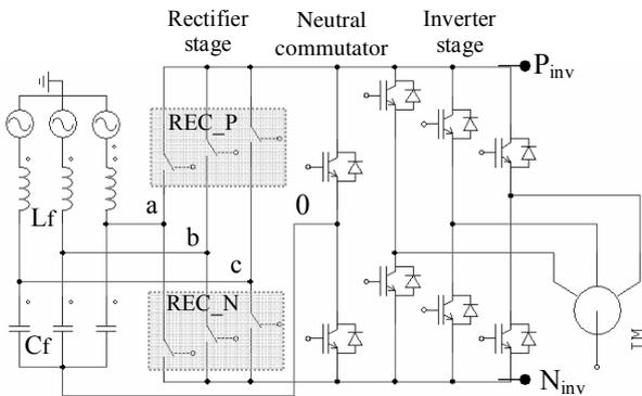
Fig. 7. Topology of a fully bidirectional three-level Indirect Matrix Converter.
