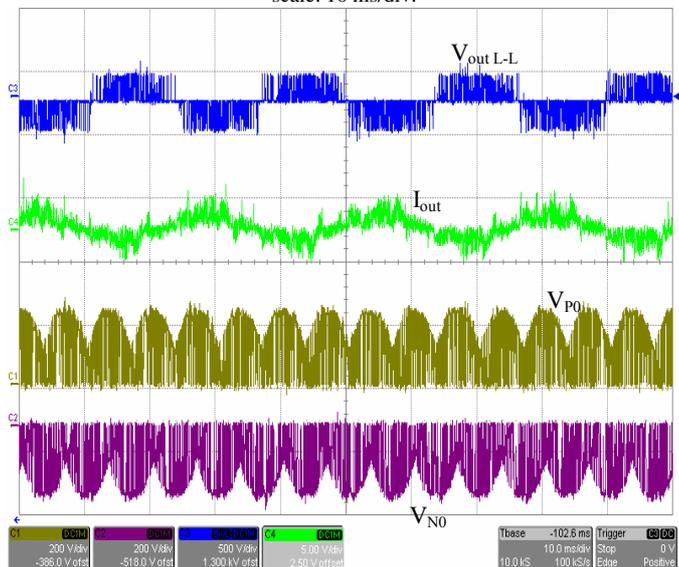
Fig. 13. Experimental results with the unidirectional three-level Indirect Matrix Converter. Waveforms (from top to bottom): the output line to line voltage  $V_{out\ L-L}$  (500 V/div); the load current  $I_{out}$  (5 A/div); the potentials of the positive  $V_{p0}$  and negative  $V_{n0}$  DC-link rail against the supply neutral (200 V/div). Time scale: 10 ms/div.
