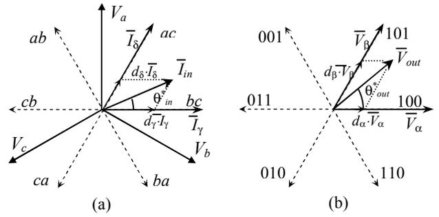
Fig. 3. Generation of the reference vectors in a two-stage Direct Power Converter using SVM: (a) rectification stage; (b) inversion stage.
