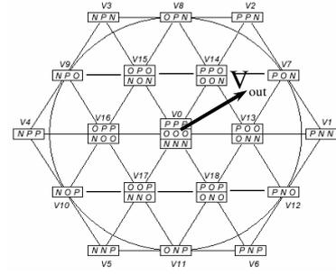
Fig. 4. Space Vector Plane for a 3-level VSI and switching
