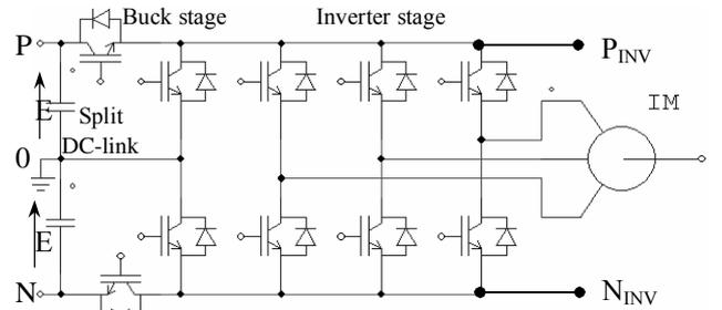
Fig. 5. Topology of the two-stage three-level buck&VSI.
