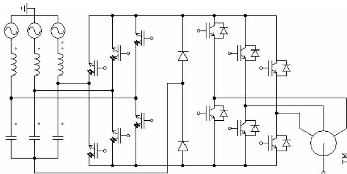
Fig. 11. Topology of the three-level Indirect Matrix Converter prototype.
