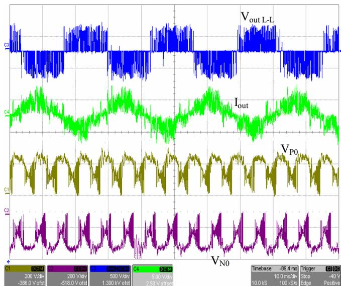
Fig. 12. Experimental results with the two-level Indirect Matrix Converter. Waveforms (from top to bottom): the output line to line voltage  $V_{out\ L-L}$  (500 V/div); the load current  $I_{out}$  (5 A/div); the potentials of the positive  $V_{p0}$  and negative  $V_{n0}$  DC-link rail against the supply neutral (200 V/div). Time scale: 10 ms/div.
