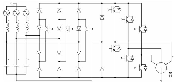
Fig. 8 Topology of a very sparse unidirectional three-level Indirect Matrix Converter using only 9 IGBTs.
