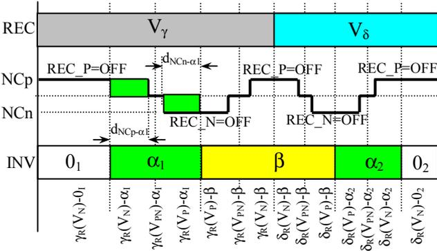
Fig. 9. Switching pattern for the 3-level Indirect MC.
