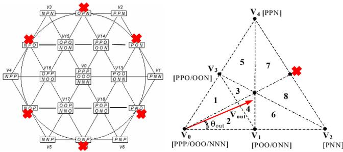
Fig. 6. a) Available switching states for the proposed two-stage/3-level VSI and b) the definition of the subsectors for SVM generation.
