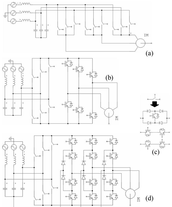
Fig. 1. Different Direct Power Converter topologies: a) standard single-stage matrix converter [1]; b) two-stage indirect matrix converter [6]; c) typical bi-directional switch implementation; d) two-stage 3-level matrix converter [7].
