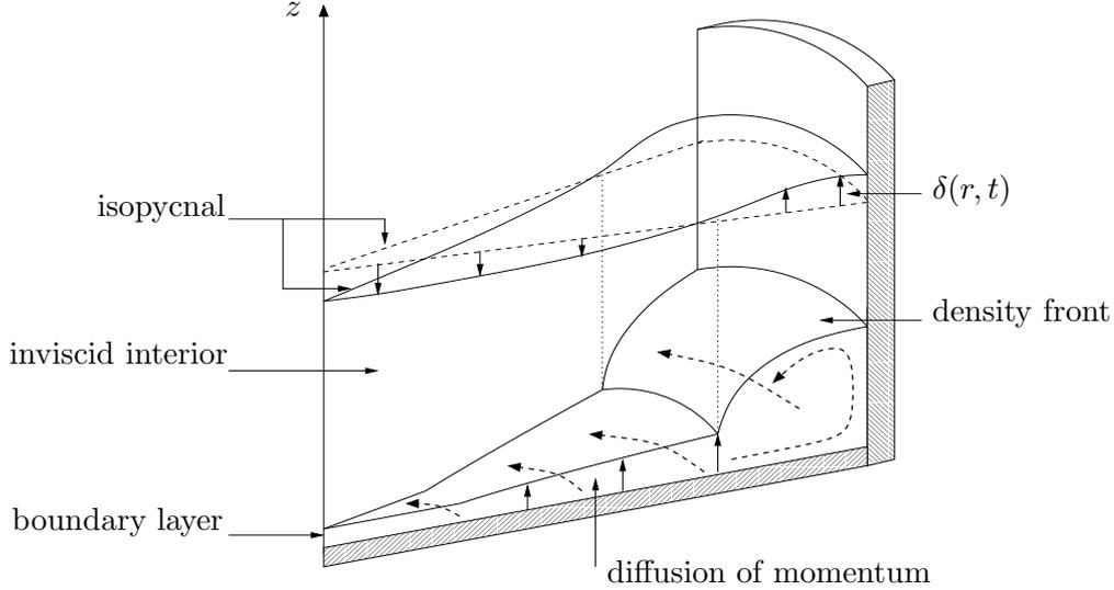
Fig. 2. Schematic diagram showing the important features of the initial flow, and the resulting effect (including the vertical isopycnal displacement  $\delta(r, t)$  - see text) on the background stable density field.
