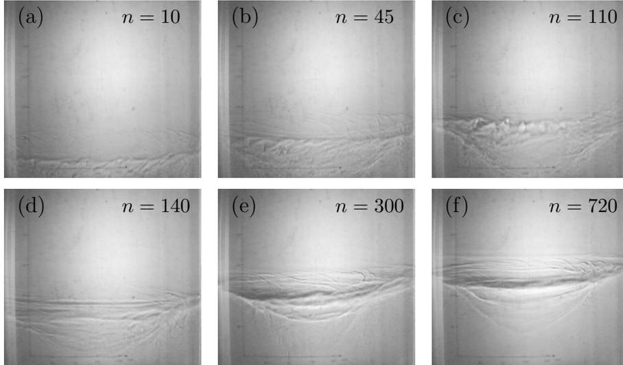
Fig. 4. Experiment I: sequence of shadowgraph images with the corresponding number of disk rotations,  $n = \omega t/2\pi$ , shown in the top right-hand corner of each image.
