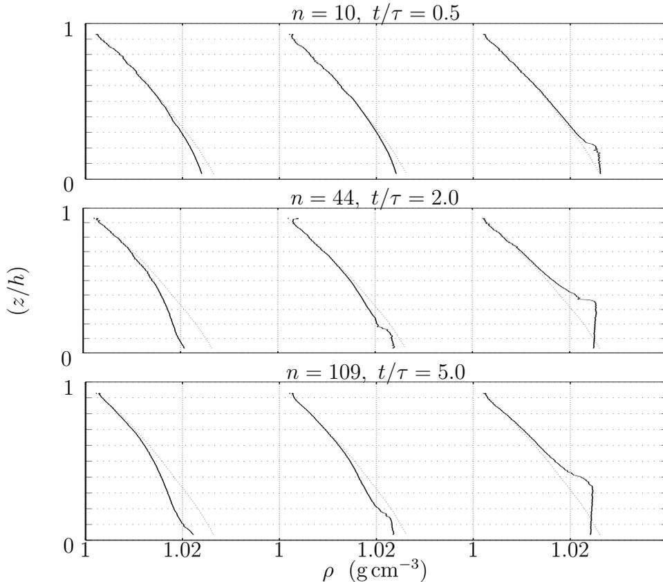
Fig. 3. Experiment I: sequence of density profiles during the early stages of the flow development, with  $\tau \approx 140$  s and  $l_z \approx 5$  cm. Each sequence consists of the three profiles obtained at radial locations  $r/R_d = 0, 0.5, 0.9$  (from left to right respectively); the corresponding initial linear profiles are also shown (dotted-lines). The horizontal density axis for the bottom plot is the same for the two above.
