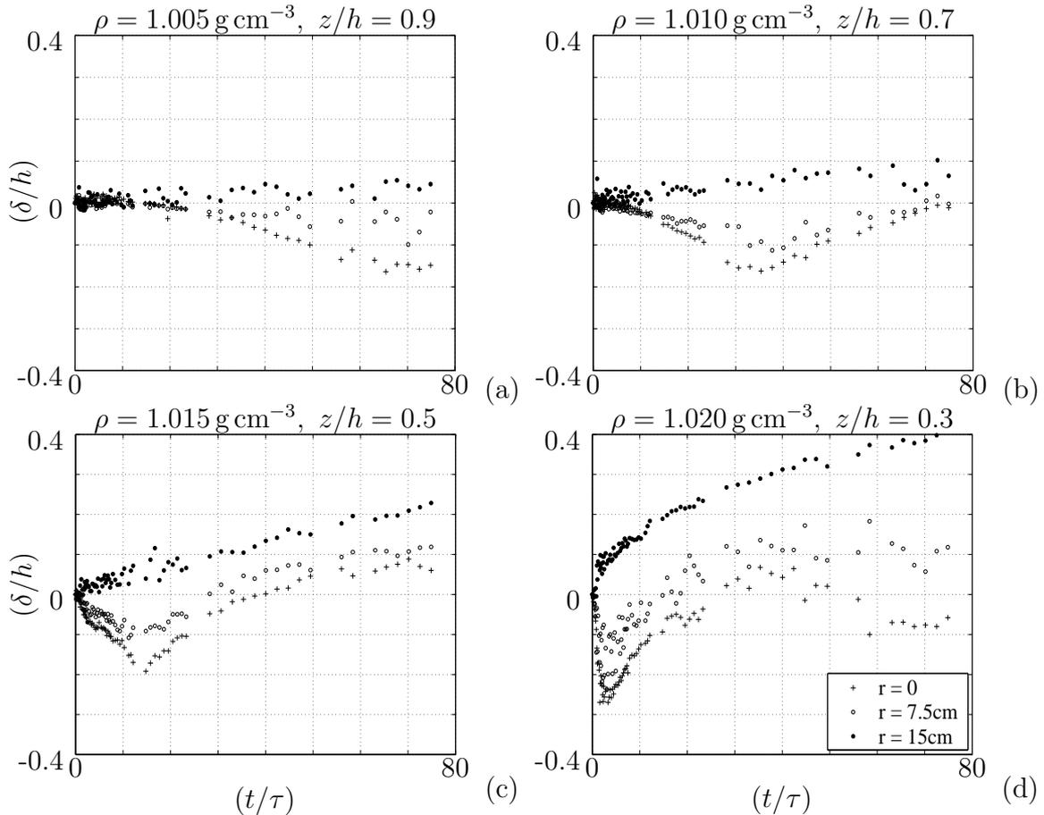
Fig. 7. Experiment I: plots showing the transient behaviour of the displacement,  $\delta(r, t)$ , of four separate isopycnals (the specific isopycnal density and corresponding initial height are shown along the top of each plot). Each plot contains three sets of measurements corresponding to the radial locations  $r/R_d = 0, 0.5, 1$ ;  $\delta(r, t)$  and  $t$  have been made dimensionless using  $h$  and  $\tau = E^{-\frac{1}{2}} N_0^{-1}$  respectively.
