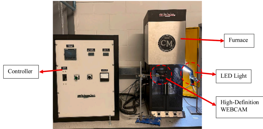
Fig. 2. A programmable bottom-loading isothermal furnace with a camera recording the live time of thermal cycling samples.
