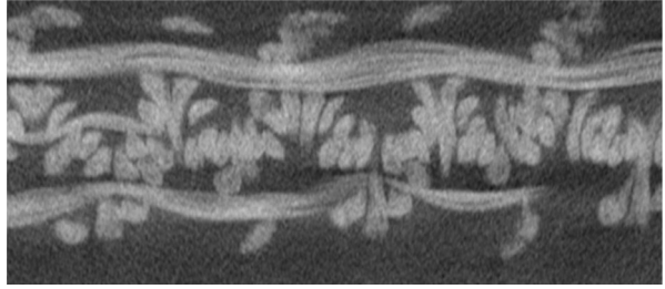
Fig. 8 CT slices from woven T-Joint, showing the weft yarn configuration at the junction region as they crossover
