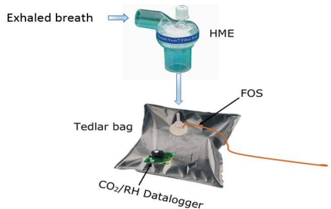
Fig. 3. Schematic experimental set-up for the breath gas measurement.
