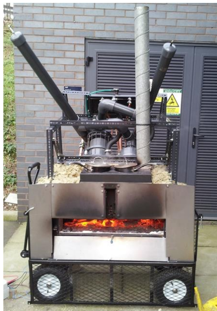
Figure 2. a) Twin core TAE prototype [28] b) Schematic of the twin core TAE.
