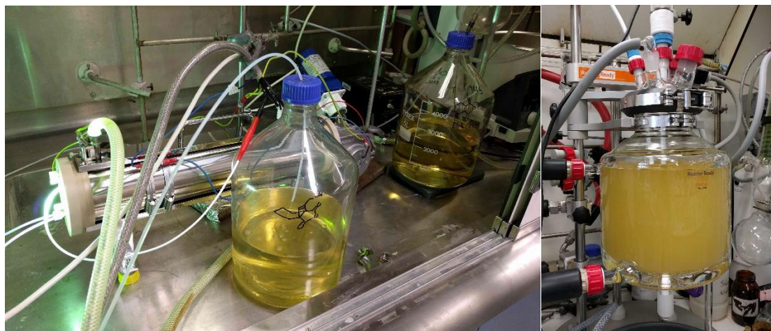
Figure S5: left – 5 mole scale irradiation of THPA with Firefly flow reactor; right – 5 mole scale hydrolysis as an emulsion
