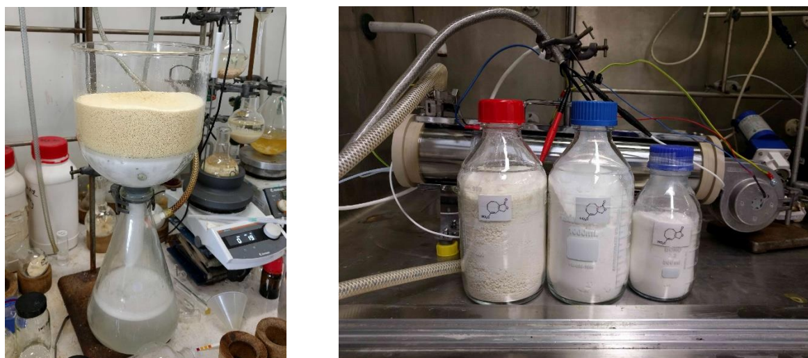
Figure S6: left – final filtration of 5 mole scale reaction; right – product batches accumulated during studies
