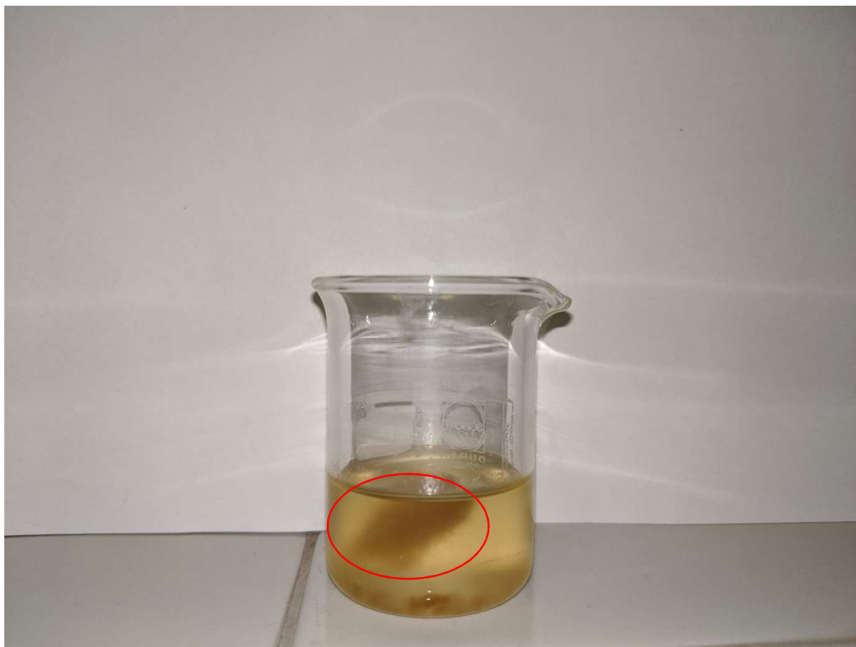
Supplementary Figure 4. Crosslinked pCHA-HMW in THF. The material produce was largely insoluble even after 72 h of constant stirring in THF (RT).
