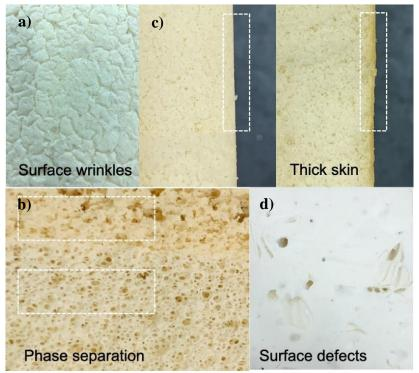
FIG. VI. Latex foam failure
