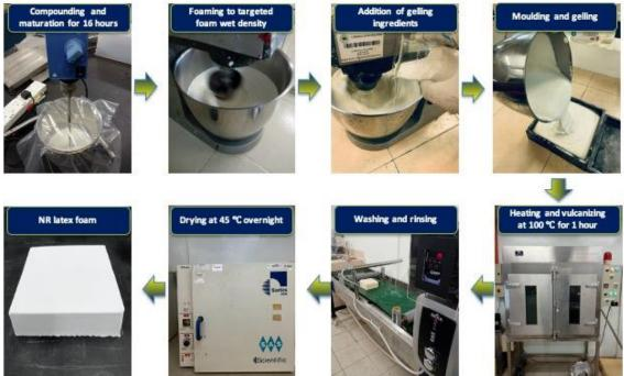
FIG. II. The different stages involved in the fabrication of NR latex foam using the Dunlop batch foaming
