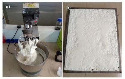
FIG. V. Failure during foaming process a) Foam coagulate; b) Foam collapse
