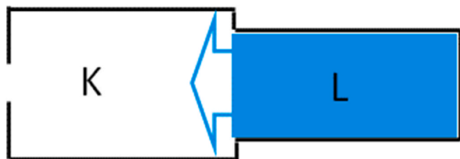
Fig. 18. Schematic diagram of the seeded percolation process. The blue shading represents the presence of liquid condensate, while regions left white represent vapour-filled pores. The arrow signifies the presence of a free meniscus from which desorption can occur in the direction shown. (For interpretation of the references to colour in this figure legend, the reader is referred to the Web version of this article.)
