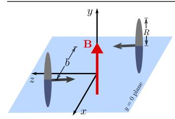
FIG. 1. A heavy-ion collision described in our coordinate system, where z is the beam axis and the impact parameter b lies along the x axis. For ultraperipheral collisions  $b \approx 2R$ . At the center of the collision, the electric fields of the two ions point in opposite directions and therefore cancel, while the magnetic fields point in the same direction and therefore double up.
