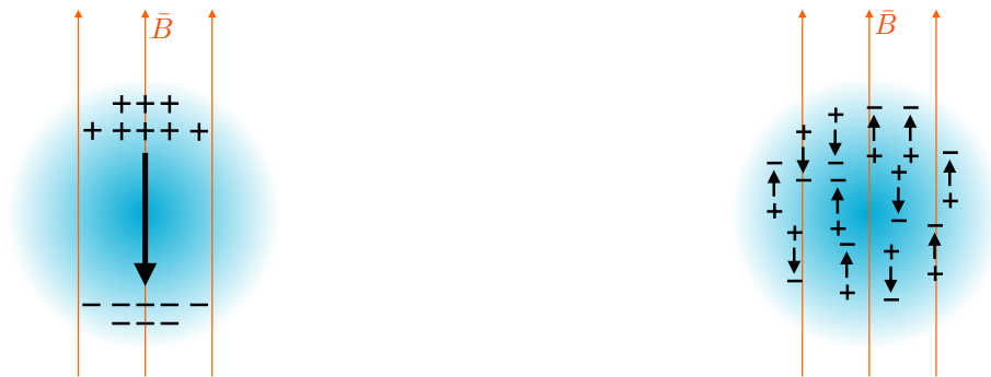
Figure 12. A soliton of the axion field in an external magnetic field creates a coherently oscillating dipole configuration, which leads to dipole electromagnetic radiation. If instead, we replace the soliton with N oscillating dipoles with random phases, we can get less power radiated than the coherent soliton case for sufficiently large N .
