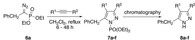
**Table 1.** 1,3-Dipolar cycloaddition of diazophosphonate **6a** to alkynes.
