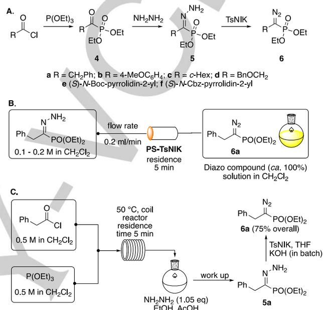
**Scheme 2.** A. Preparation of diazophosphonates **6** by oxidation of hydrazones **5**; B. Flow preparation of diazophosphonate **6a**; C. Flow preparation of hydrazone **5a**, and its subsequent oxidation to diazophosphonate **6a**.
