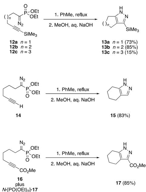
**Scheme 6.** Intramolecular cycloaddition of diazophosphonates to alkynes to give cycloalkapyrazoles.
