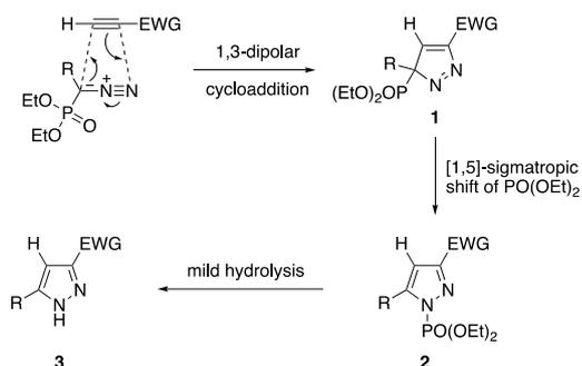
**Scheme 1.** Diazophosphonates in pyrazole synthesis (EWG = electron-withdrawing group)
