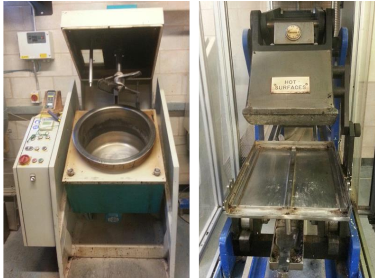
Fig. 2. (a) Mixer, and (b) Steel roller
