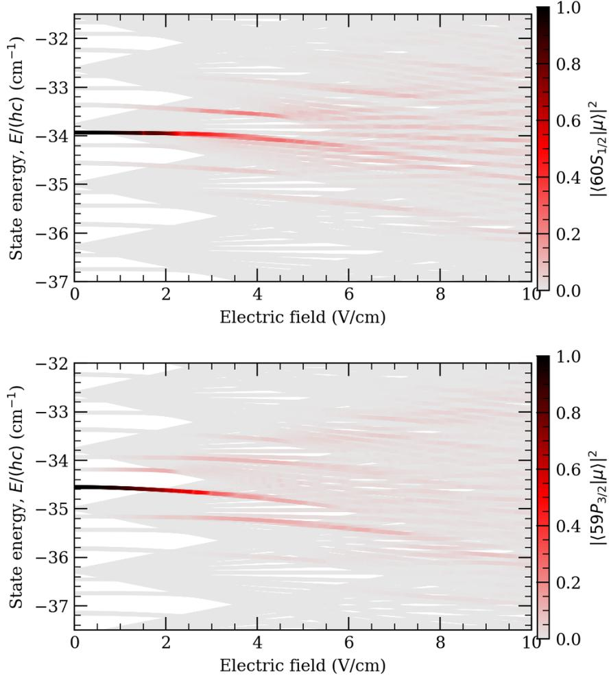
Figure S3: Stark shifts of the  $60S_{\frac{1}{2}}, 59P_{\frac{3}{2}}$  energy level of Rubidium. The stark effect is only quadratic for small  $E_0$ . Divergence from a simple  $E^2$  relationship begins at around around  $E_0 = 2$  V/cm, and is clearly present at  $E_0 = 4$  V/cm for both states. This effect can be seen in the divergence of the observed fringe visibility from the quartic model of figure (S2).
