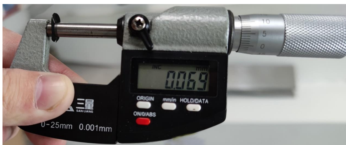
Figure S6. Digital photo of CAC-1 electrode with PTFE binder.
