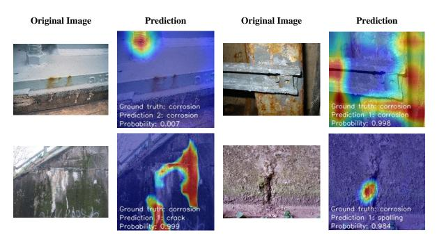
Figure 6: VGG16 trained on corrosion, crack, and spalling classes. Top row: images are correctly classified using incorrect features. Bottom row: defect features are correctly identified, however the predictions are scored as "incorrect" due to poor ground truth labels.
