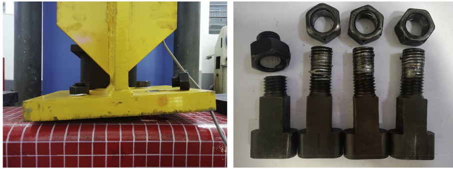
(b) TSOB Bar fracture
