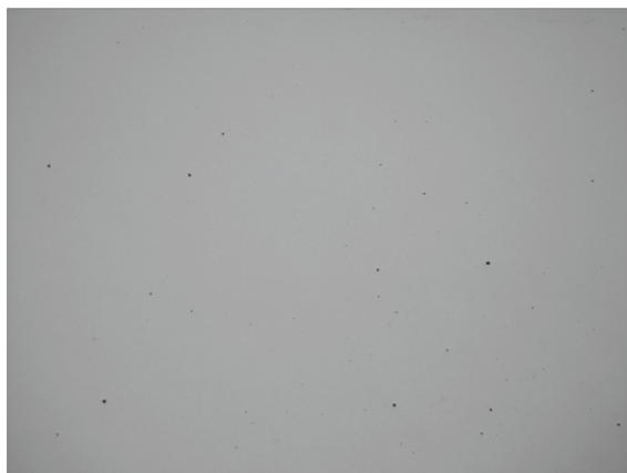
Fig. 4 a Original image obtained from printed nickel-based superalloy cube with porosity shown by dark spots. b Black and white image with porosity labelled as white pixel using CCL
