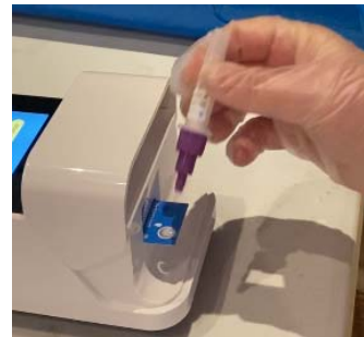
Fig. 2 The operator applies the extracted sample from the extraction vial onto the sample application area of the inserted test strip.
