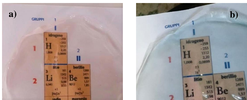
Figure 7. Thermochromic polymeric film [N_{1.13GA8}]Br/Co(NTf_2)_2/PMMA (3:1) (390 mg): a) 25 °C; b) 80 °C.
